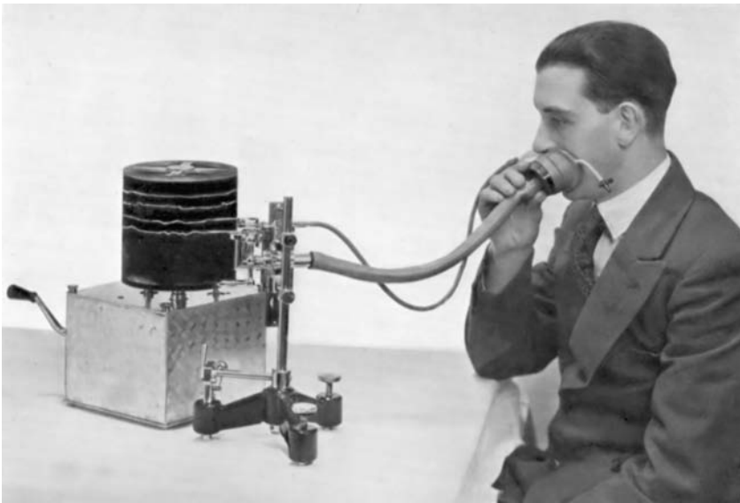
Figure 2. Edward Wheeler Scripture's kymograph, which took simultaneous recordings from the nose and mouth. Reprinted with permission from E. W. Scripture, "Registration of Speech Sounds," Journal of the Acoustical Society of America 7 (1935): 140. Copyright 1935, Acoustical Society of America.
