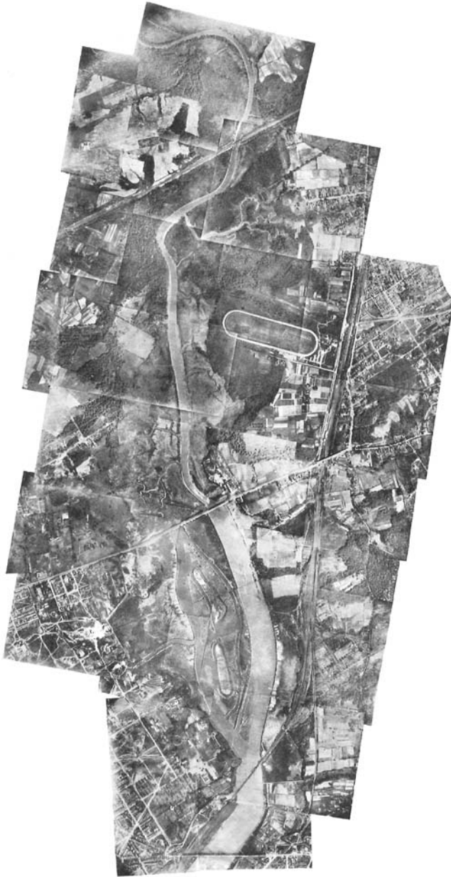
Figure 1 Photomosaic made in 1920 of land along the Anacostia River east of Washington, DC. To illustrate the method of photomosaic composition, the edges of the composite image have been left untrimmed and the variation in the constituent images' exposure uncorrected.
