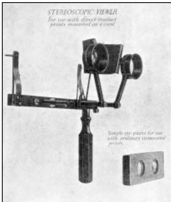
Fig. 9. Stereoscopic viewer and eyepieces, as used in World War I reconnaissance (N).
