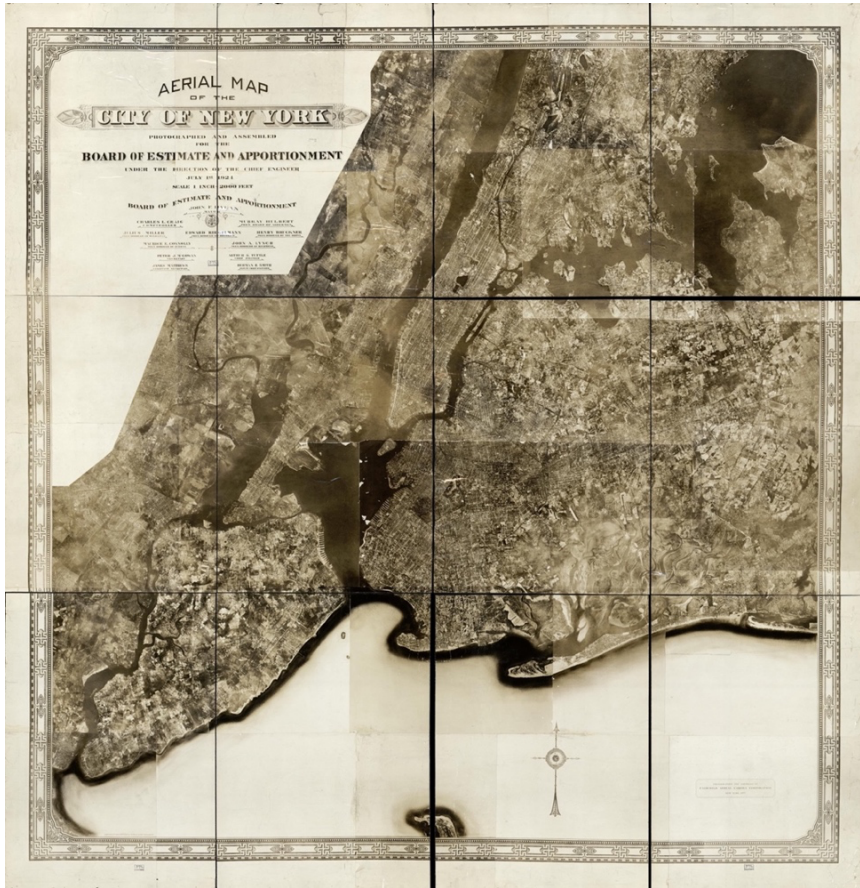
Figure 2. Aerial photomosaic of the greater New York area made by Fairchild Aerial Camera Corporation in 1924. The image was assembled from 2000 individual images taken by three planes over the course of several months.
